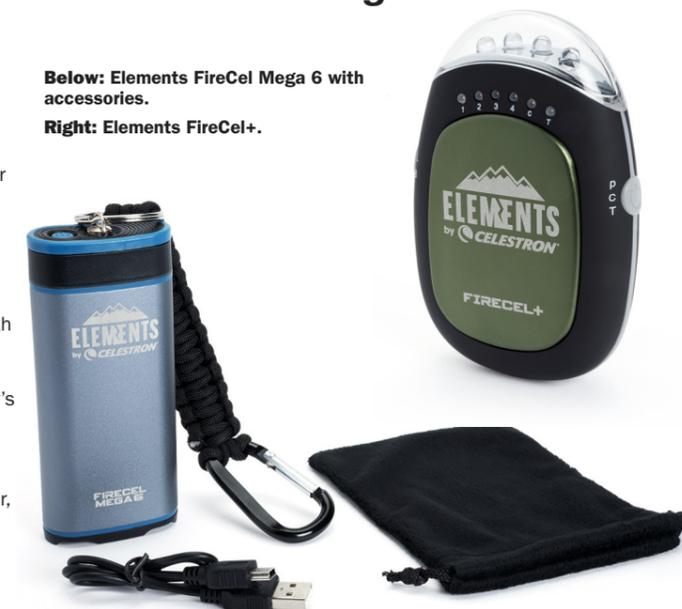
The integral flashlights comprise separate red and white LEDs and operate in five (FireCel+) or four (FireCel) different modes, including constantly flashing Morse code S-O-S for emergency situations. Connecting via each unit's USB port, I was able to successfully charge my iPhone and my small Nikon compact camera, which I use for digiscoping. Both devices have the capacity to deliver two full smartphone charges before needing to be fully charged themselves.
